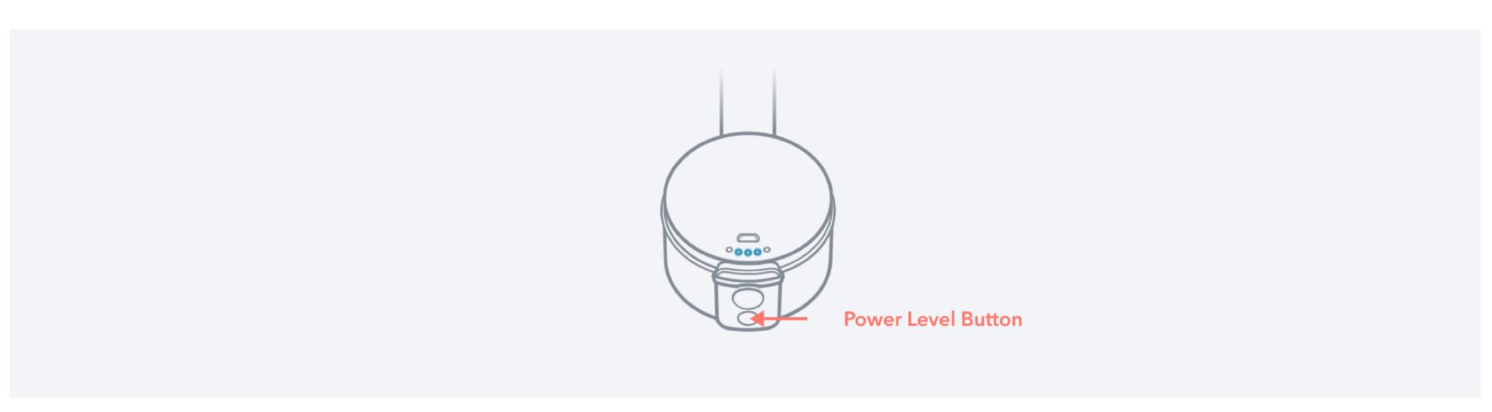
Click and release the Power Level button (small button on bottom) to select User desired Power Level. Each single button click cycles through 1 incremental Power Level, each of which represent dynamically preset temp settings:
