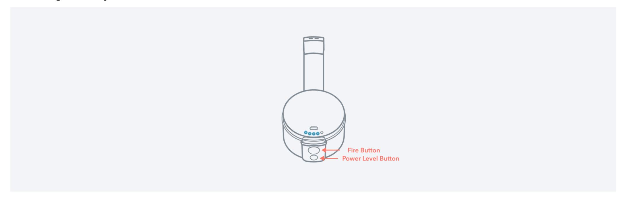
Click and release both the Fire and Power Level Button together at once to check the Puck Base Unit battery level.
