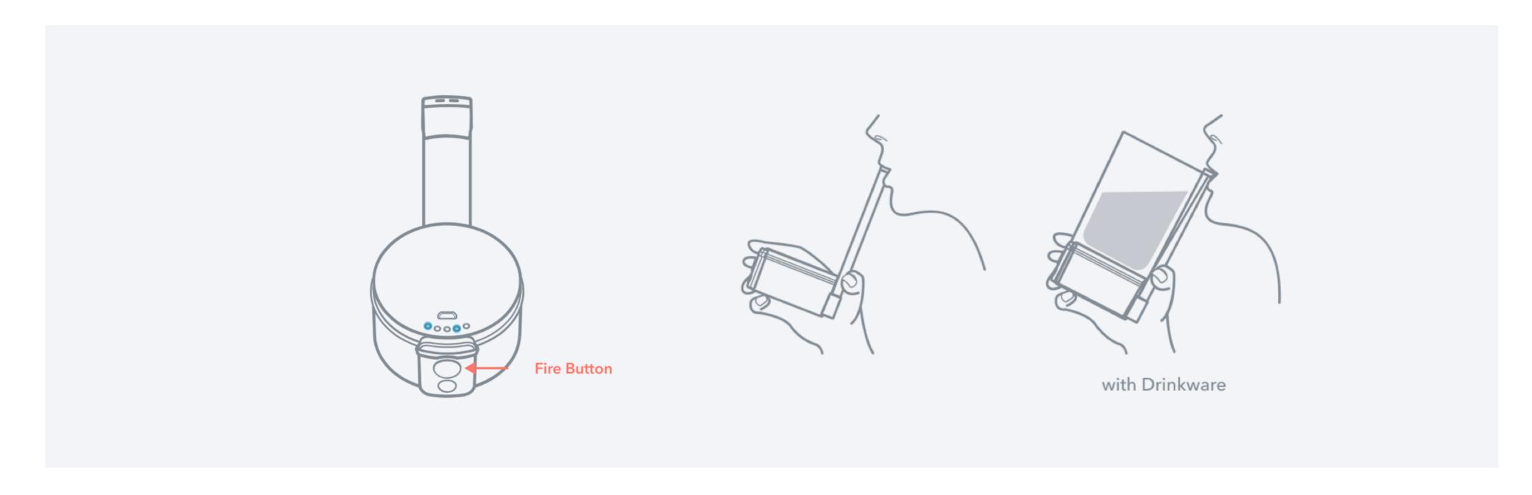
After selecting the desired power level with the Power Level select button c (small lower button), click and release the Fire button (large top button) once.
