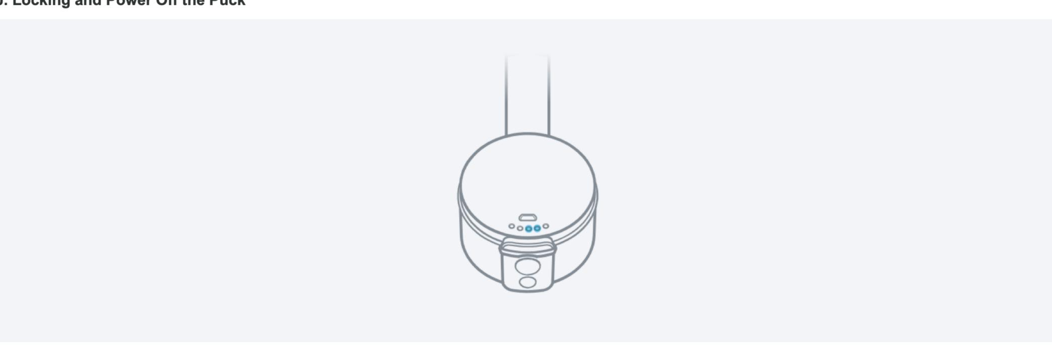
To shut down and lock the puck base unit. The User must click the Fire button 3 or more times with less than 0.3 second gap between clicks.
