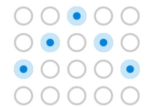
Light Blue LEDs comes on in 0.5 seconds, two inner LEDs flash blue once, then two outer LEDs flash blue, the flashing sequence repeats once more, indicating the Puck Base Unit is unlocked and ready to operate.
