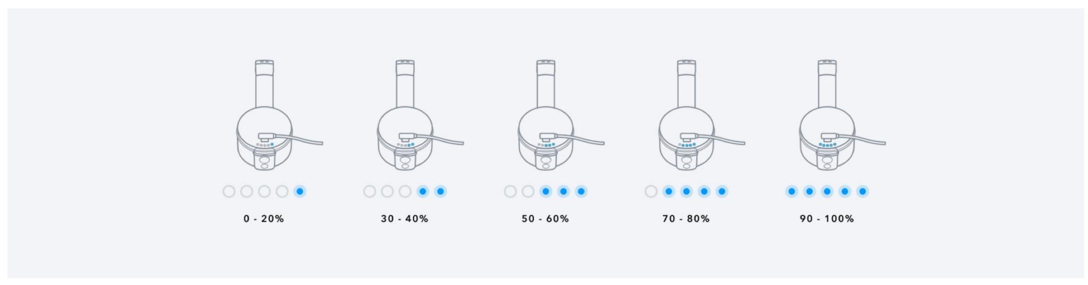
When the User plugs in the Puck to charge, its battery charging level is indicated with pulsing BLUE LEDs. (Depending on the state in which the Puck Base unit is plugged in to charge, it could take up to 10 seconds for Bowle to indicate its charging status).
